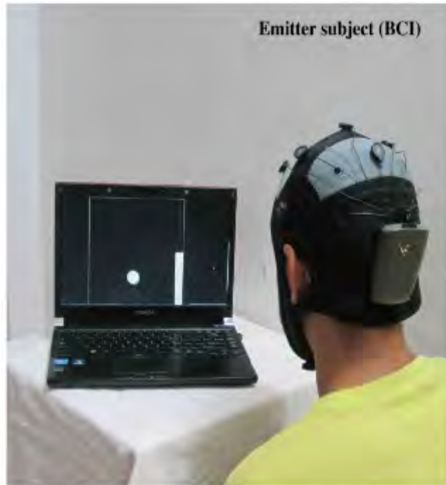
Figure 2. View of emitter and receiver subjects with non-invasive devices supporting, respectively, the BCI based on EEG changes driven by motor imagery (left) and the CBI based on the reception of phosphenes elicited by a neuronavigated TMS (right) components of the B2B transmission system. The successfully transmitted code in the particular scenario shown is a '0': the target and ball are at the bottom of the screen (correctly encoding a 0 through motor imagery of the feet) and the TMS coil is in the orientation not producing phosphenes for this particular participant (subject 2, see Figure 3), with the handle pointing upwards. doi:10.1371/journal.pone.0105225.g002
